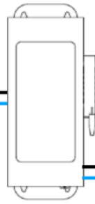
DISCONNECT SHOULD BE USED IF YOUR RUN IS OVER 50 FEET
